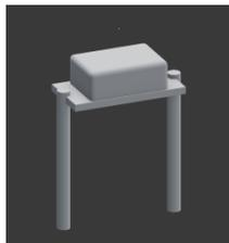
Before the wires are threaded into the tube of the post, it is worth testing whether the soldering was successful and whether the LED was not burnt. It's also worth checking the polarity and marking the ends of the wires with some colour (the green arrow on the bottom of the LED indicates the negative pole). With reversed polarity, the LED will not light up, but will not suffer any damage. However, be sure to use the proper serial resistor during the test!
